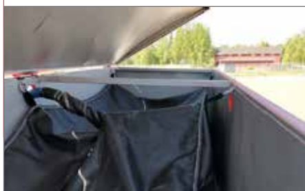
Geotextile bag effectively separates solids from water.
